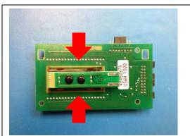
Figure 2 - Remove the old PPU backlight by squeezing the top and bottom edges while tipping the backlight towards you.
