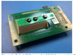
Figure 4 - Reinstall the new backlight be reversing the process shown in Step 2.
