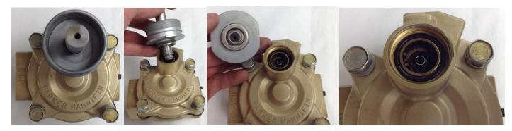
4. Remove lower plunger & spring assembly, upper plunger, upper plunger seal, upper spring, and flange O-ring.
