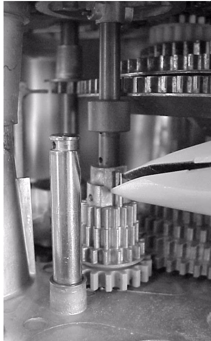
LIFT SPACER AND INSTALL VERTICAL PIN
