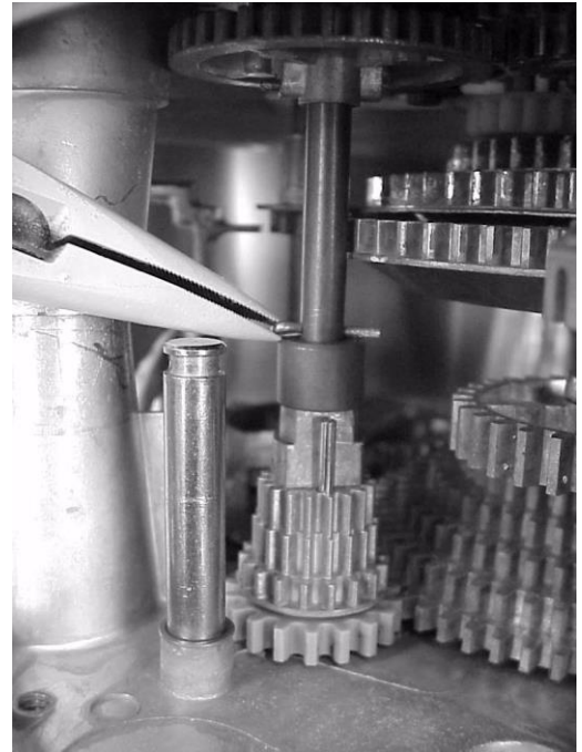
LOWER SPACER AND RE-INSTALL COTTER PIN
