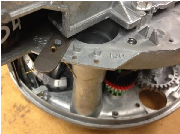
Move the Dollar Shift Lever to the "100" position (the RIGHT most stud)
