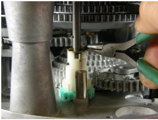
G. Reseat the washer on top of the gear and reinsert the cotter pin.
