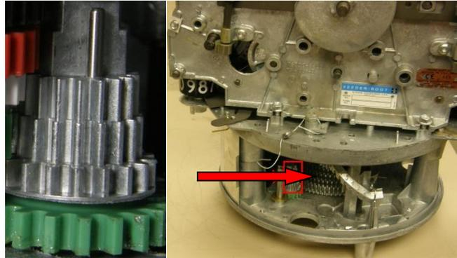
**Figure 2b – Dollar Dive Shaft Gear Location**
