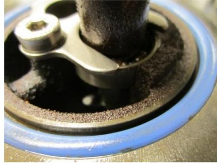
Close-up with head removed showing ULSD debris
