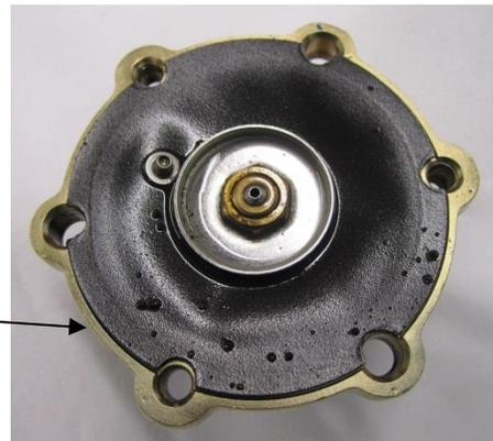
Close-up of valve diaphragm showing ULSD debris
