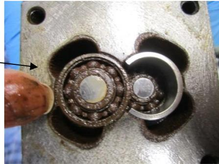
Close-up with end cap removed showing ULSD debris
