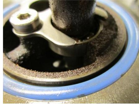
Close-up with head removed showing ULSD debris
