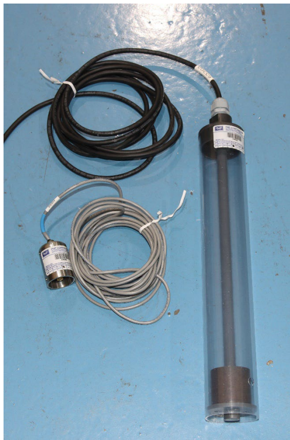
Figure 1: Test Unit Sensors Sent by PMP, The Shorter Sensor is Type 63304, The Tall Sensor is Type 63303.
