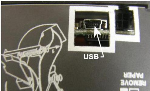
Re-establish the USB connection after an interruption of about one (1) minute in order to re-activate the driver software.
