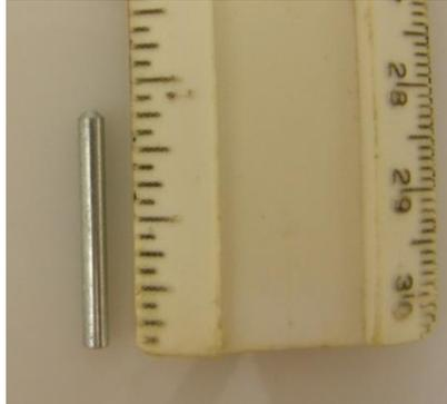
**Figure 2a – Dollar Drive Shaft Pin**
