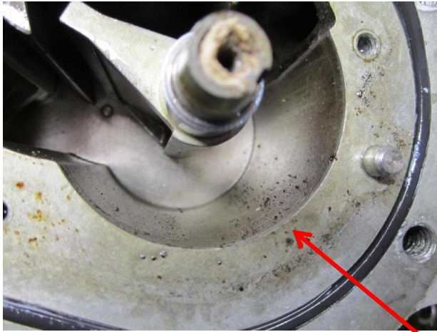
Particles that caused meter to lockup
