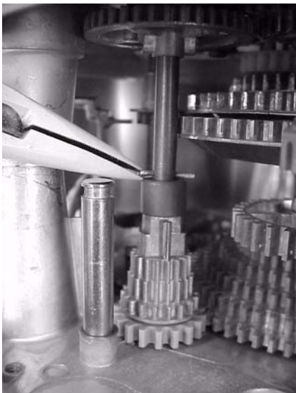
Remove cotter pin above spacer
