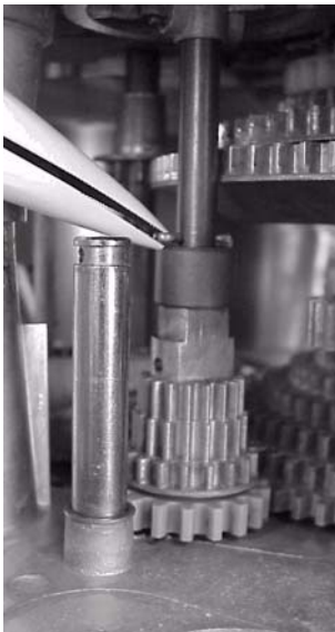
Lower spacer, re-install cotter pin
