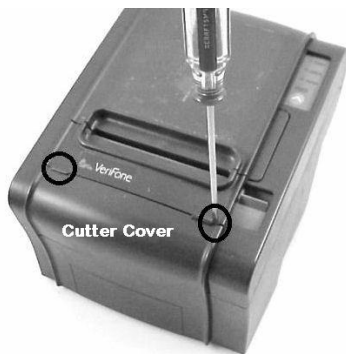
No. 1 Gently prying Cutter Cover off
