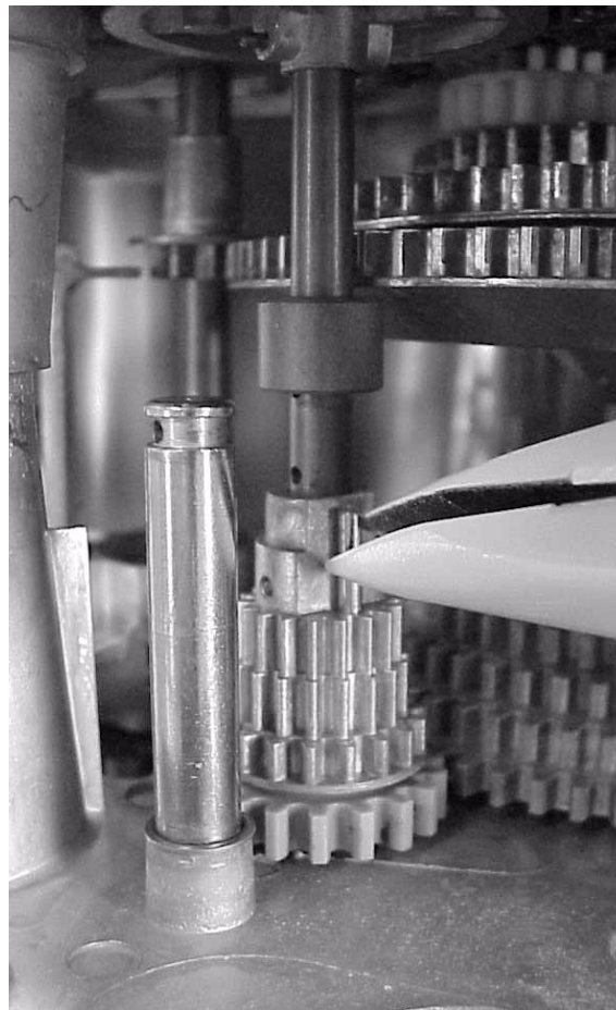
LIFT SPACER, INSTALL DOLLAR DRIVE SHAFT VERTICAL PIN
