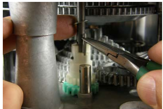
F.) Slide the washer up the dollar drive shaft and insert the dollar drive shaft vertical pin (you will need to rotate the gear to get the pin to seat into the bottom gear).
