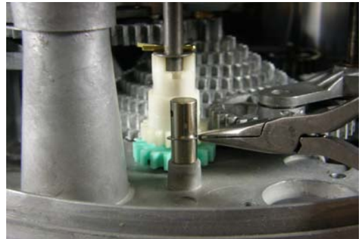
D.) Remove and save the bottom washer which has an outer diameter of 5/16".
