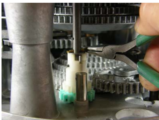
G.) Reseat the washer on top of the gear and reinsert the cotter pin.
