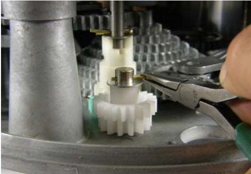
A.) Locate the white plastic compound gear and remove and save the cotter pin.
