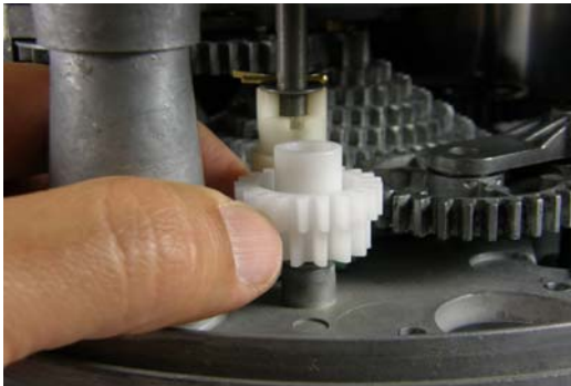
C.) Remove and save the white plastic compound gear.
