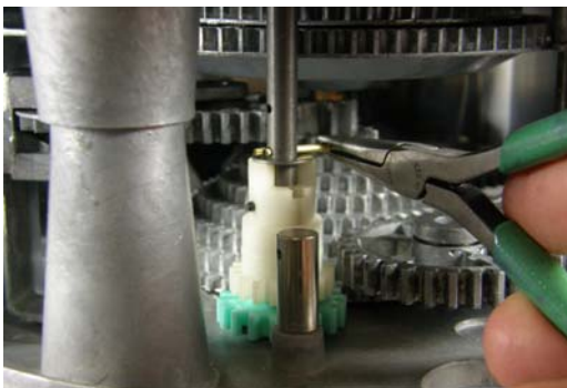
E.) Remove the cotter pin from the dollar drive shaft.
