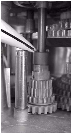
Lower spacer, re-install cotter pin
