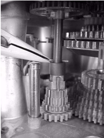
Remove cotter pin above spacer
