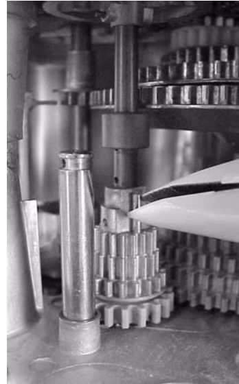
Lift spacer, remove Dollar Drive Shaft Vertical Pin
