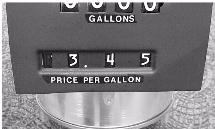
Example of Price-Posting Wheels Showing $3.45 (Leftmost (Small) Wheel is in the “Blank” Position)
