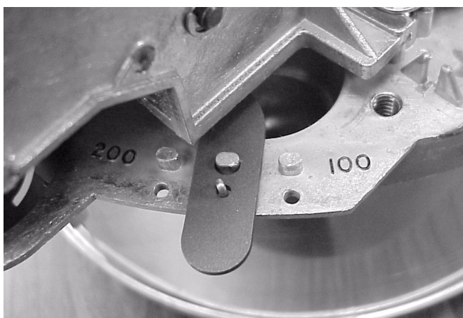
Dollar Shift Lever in Central Position
