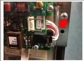
Figure 6 - Dress the Backlight and Thermistor cable
