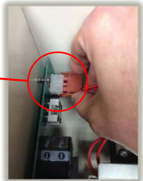
Figure 3 – Squeeze the two tabs to un-plug the power connector
