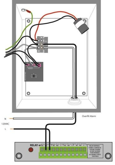
Sample TLS-350 wiring for 4-Relay Output Module
